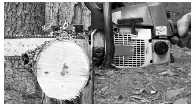
\* When cutting with the log holder always cut with the wood resting against the housing. Wood lengths should have clean cut ends. Do not overload the log holder.
